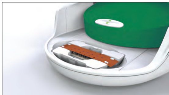
Fig. 2.5. Loaded DG8 Cartridge placed in the QX200 Droplet Generator.
