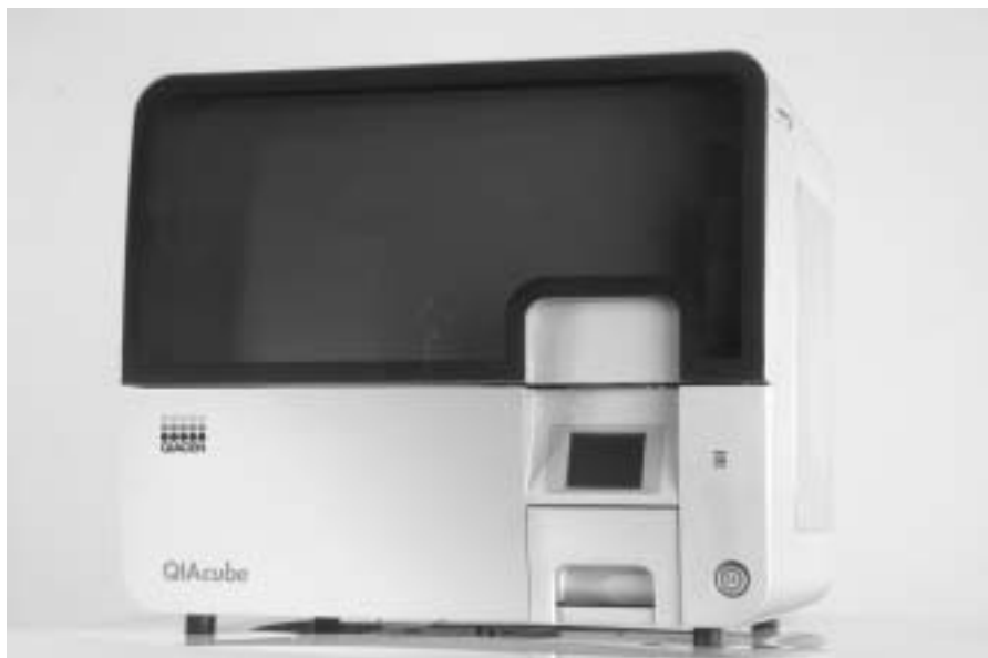
Figure 1. Automated DNA purification. DNA purification using the QIAamp DNA Mini Kit or the QIAamp DNA Blood Mini Kit can be fully automated on the QIAcube.
